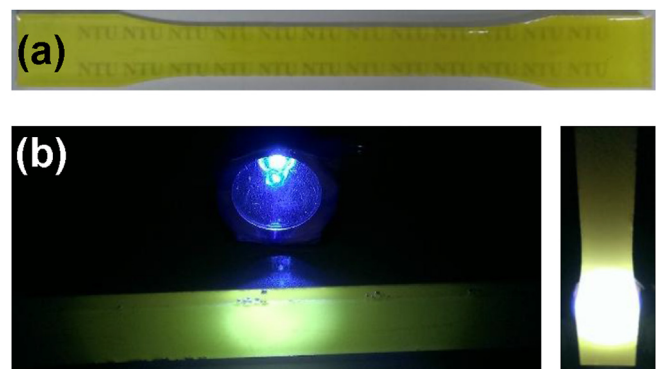
Fig. 10. (a) Cured film at MMT-POP2000-70:YAG:anhydride/epoxy = 1:5:100 by weight and (b) light emitting test for the film.
